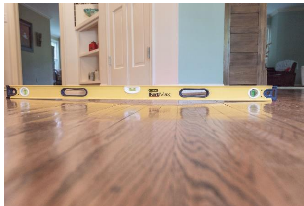
An easy way to visually test for a sagging floor is to put a level above the area you suspect is sagging.
